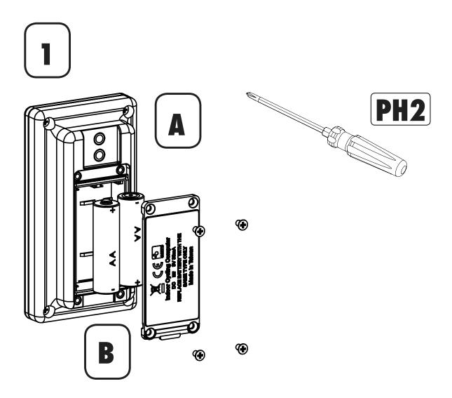
The use of rechargeable batteries may lead to malfunction of the console unit due to a voltage lower than 1,5 V.
